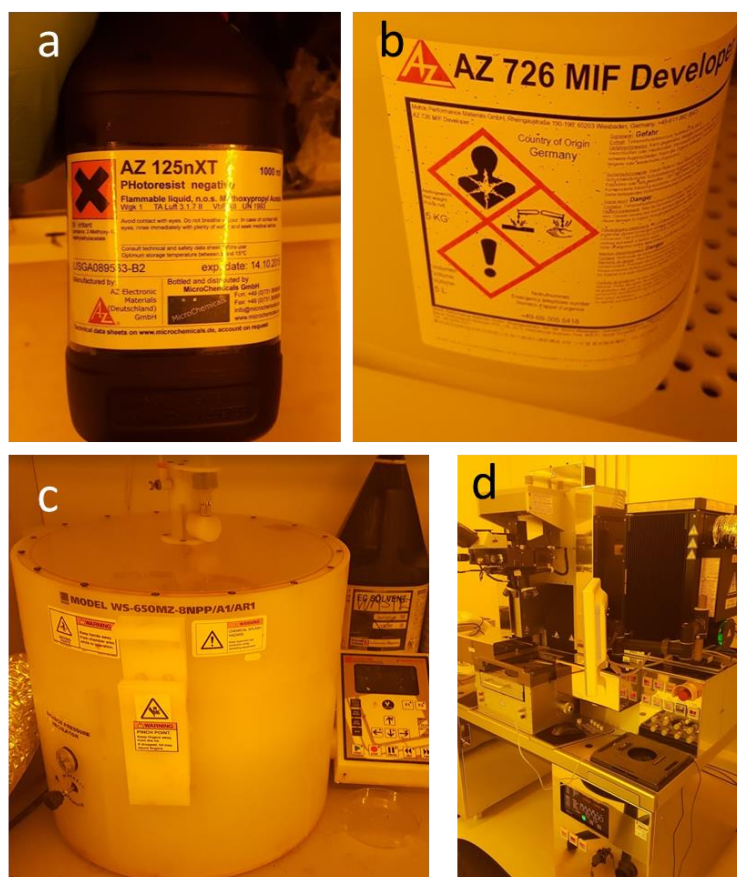
Figure 3.14 Photolithography chemicals and equipment. (a) A cross-linking negative photoresist AZ® 125 nXT (MicroChemicals), (b) AZ 726 MIF developer, (c) Model WS-650MZ-8NPP Spin Coater (Laurell Technologies), (d) Suss MicroTec MA8 contact mask aligner.
