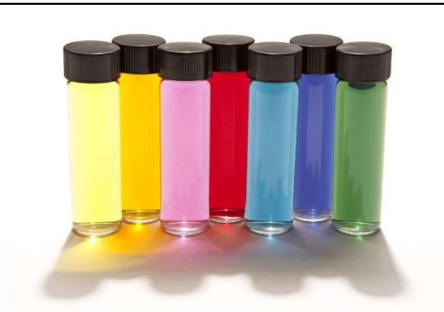
Figure 2.12. Colloidal metallic nanoparticles generating colour through their plasmonic resonance [35].
