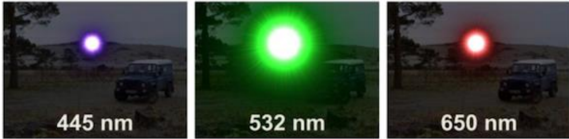
Figure 2.35. Visual dazzle resulting from difference laser wavelengths of equal irradiance at dusk/dawn conditions [75].
