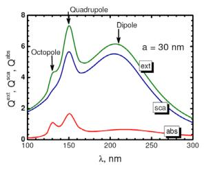
Fig. 2. Inverse hierarchy of resonances for an aluminum particle in vacuum. Normalized extinction, scattering and absorption cross-sections,  $Q^i = \sigma^i / \pi a^2$ , for a particle with a = 30 nm as functions of incident light wavelength  $\lambda$ . Points of dipole, quadrupole and octopole resonances are indicated with arrows. The extinction cross-section of the quadrupole resonance is the greatest. With a = 40 nm the octopole resonance becomes the greatest [11].
