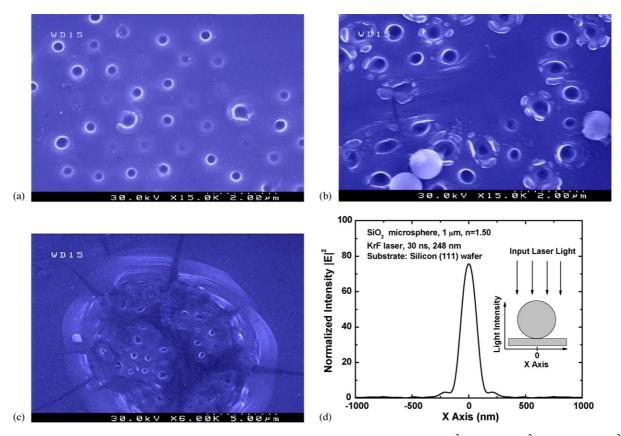
Fig. 2. SEM images of Si(111) wafer patterned with SiO<sub>2</sub> microsphere mask at laser fluences of (a) 100 mJ/cm<sup>2</sup>, (b) 160 mJ/cm<sup>2</sup> and (c) 240 mJ/cm<sup>2</sup>. (d) The calculated intensity of the laser light on the silicon surface. The intensity  $E^2$  is normalized to input intensity  $E^2_0$ .
