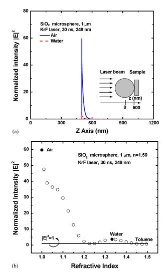
Fig. 4. Results of near-field optical calculations of laser irradiation of a SiO<sub>2</sub> microsphere on 35-nm silver film. (a) Normalized optical enhancement along the z axis; (b) normalized optical enhancement under SiO<sub>2</sub> microsphere in different media. The intensity  $E^2$  is normalized to input intensity  $E^2_0$ .
