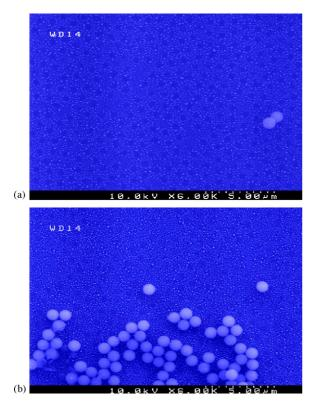
Fig. 3. SEM images of (a) 35-nm silver films patterned with  $SiO_2$  microsphere mask in air, and (b) in water. The laser fluence was 240 mJ/cm<sup>2</sup>.
