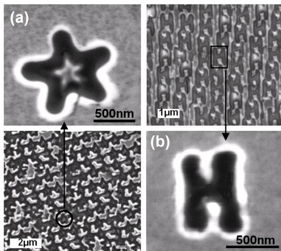
**Figure 4.** SEM images of star-shape arrays (a) and H-shape arrays (b) produced by scanning beams with designed angles
