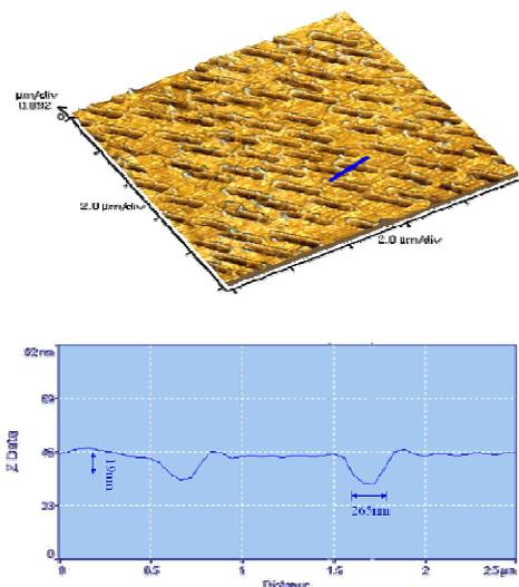
**Figure 3.** AFM profile of ordered arrays of line structures, fabricated by ALBS technique.
