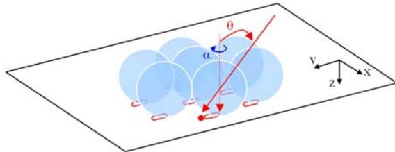
**Figure 1.** Schematic diagram of the experimental configuration for direct laser writing of nano-line arrays on substrate surface
