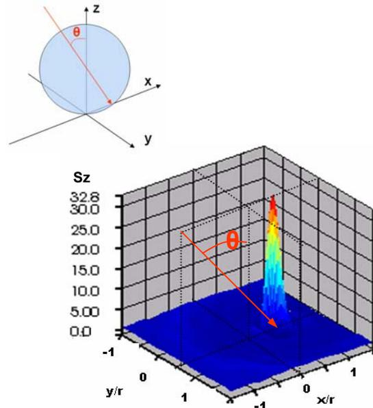
**Figure 2.** Calculated Poynting intensity distribution  $S_z$  for  $\lambda = 248\text{nm}$  radiation with incident angle ( $\theta=30^\circ$ ) under a  $\text{SiO}_2$  sphere ( $n = 1.51$ ) of radius ( $r=500 \text{ nm}$ ) on  $\text{SbTe}$  substrate ( $n = 1.80, k = 2.07$ ).
